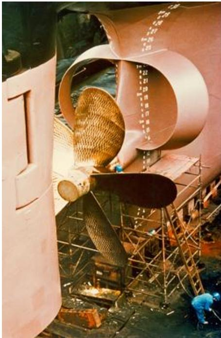
**Figure 9.2 – Typical wake equalising duct** [Scheneekluth]
