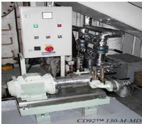
**Figure 9.11 – Typical homogeniser**
