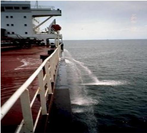
**Figure 4.3: Ballast water exchange using flow-through method** [Wikipedia]
