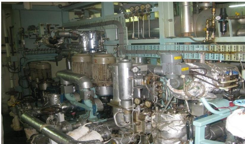
**Figure 7.5 – Viscosity controller and fine filter units**
